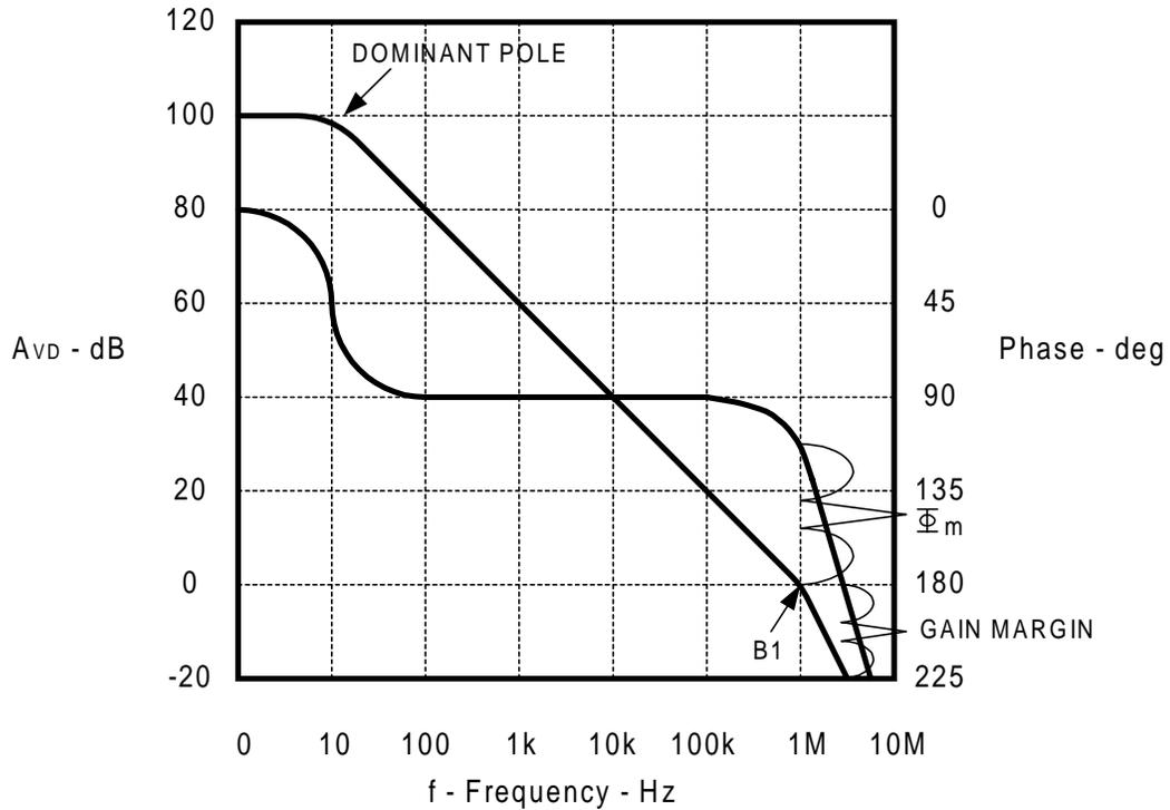
Figure 18. Easier to Read Graph of Voltage Amplification and Phase Shift vs. Frequency
