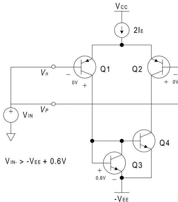
Structures like the one shown in the example above do not allow the common-mode input voltage to include either power supply rail. Other technologies used to construct op amp inputs offer different common-mode input voltage ranges that do include one or both power supply rails. Some examples are as follows (reference schematics can be found in the Texas Instruments' data book, *Amplifiers, Comparators, and Special Functions*):
