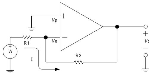
To understand this circuit, we must derive a relationship between the input voltage,  $V_i$  and the output voltage,  $V_o$ .
