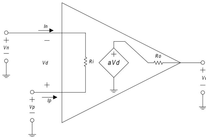
We still have the loading effects at the input and output ports as noted above. The ideal op amp model was derived to simplify circuit calculations and is commonly used by engineers in first-order approximation calculations. The ideal model makes three simplifying assumptions:
