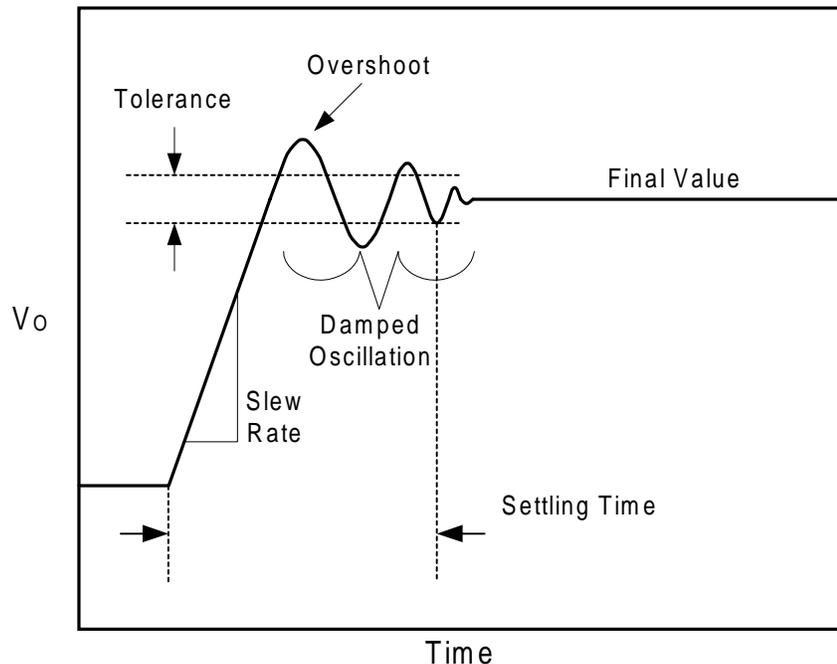
Settling time is a design issue in data acquisition circuits when signals are changing rapidly. An example is when using an op amp following a multiplexer to buffer the input to an analog to digital converter. Step changes can occur at the input to the op amp when the multiplexer changes channels. The output of the op amp must settle to within a certain tolerance before the analog to digital converter samples the signal.
