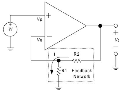
To understand this circuit we must derive a relationship between the input voltage,  $V_i$ , and the output voltage,  $V_o$ .
