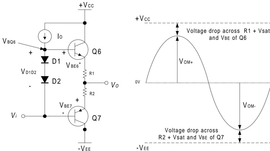
The maximum value that  $V_{BQ6}$  can be is  $+V_{CC}$ , therefore  $V_O \leq +V_{CC} - V_{R1} - V_{BEQ6} - V_{SATQ6}$ . The minimum value that  $V_i$  can be is  $-V_{EE}$ , therefore  $V_O \geq -V_{EE} + V_{R2} + V_{BEQ7} + V_{SATQ7}$ .
