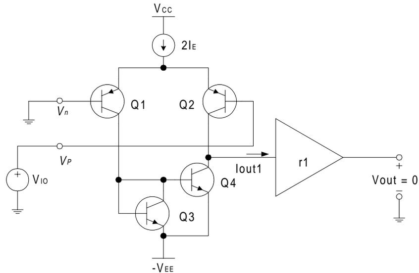
Input offset voltage is of concern anytime DC precision is required. Several methods are used to null its effects.
