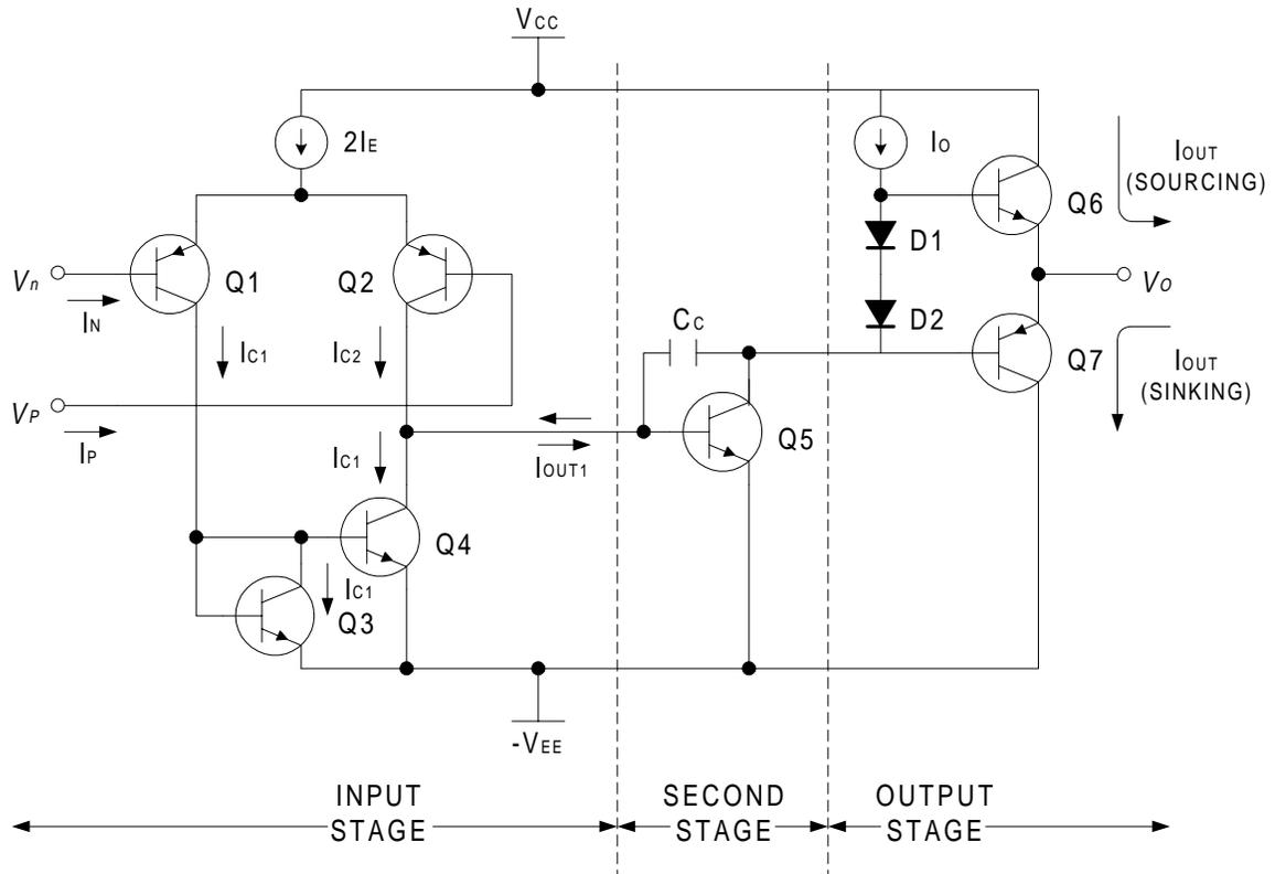
Although simplified, this circuit contains the three basic elements normally found in op amps:
